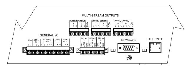
Figure 4-6: Rear Panel Electrical I/O Connections
